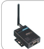
NPort® Z2150 Series 1-port RS-232/422/485 serial-to-ZigBee converters
