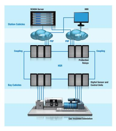
In the 1960's a conventional substation was rather bulky, with copper or fiber wiring used to hard-wire The release of the IEC 61850 Station Bus protocol in the 1980's was a big first step forward on the way to implementing a substation-wide all-purpose network.
