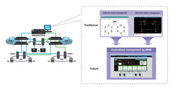
Sometimes substation networks deploy switches that do not have integrated IEC 61850 MMS, making network management more complex as these switches cannot be integrated easily into the PSCADA system. Moxa's network management software supports RESTful APIs and web widgets that enable easy integration of such devices with third-party applications (e.g., web-based SCADA).
