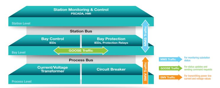
The example in the following figure illustrates how the three protocols contribute to substation communication.
