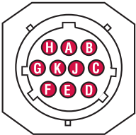
Male, 10-pin (MS) integral connector (pin-out as viewed from the end of the sensor)
