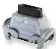
Upper housing BAS GOT16 FCS ZH V; with **podis** flat cable feed-through, for two-hand locking; degree of protection IP65; color: silver gray RAL 7001
