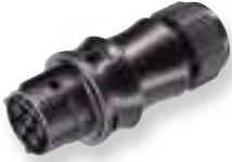
Pluggable connector RST 20i5, 5 pole, screw-in socket part, 250/400 V, 20 A, for cable diameter 6-10 mm, black color coding, black housing color; for rigid, for fine-stranded and multi-stranded cables from 0.75 to 4 mm<sup>2</sup>; Degree of protection IP65, IP66, IP67, IP68 (3 m, 2 h); unassembled with cable screw connection and locking, UL/CSA;
