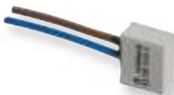
Surge protection AS-i and DC 24 V, surge protection for DC 24 V and AS-i in a cup, potted; against over-coupling during switching operations or short circuits, features: for in-plug installation, connection modules
