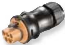
Pluggable connector RST 20i4, 4 pole, screw-in plug part, 50 V, 20 A, for cable diameter 6-10 mm, brown color coding, black housing color; for rigid, for fine-stranded and multi-stranded cables from 0.75 to 4 mm<sup>2</sup>; unassembled with cable screw connection and locking
