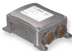
RST compact distributor RST 20i4, 4 pole, 1 input, 3 outputs, with fixing option, AS-i/24V, 20A, brown color coding
