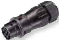
Pluggable connector RST 20i5, 5 pole, screw-in socket part, 250/400 V, 20 A, for cable diameter 13-18 mm, black color coding, black housing color; for rigid, fine-stranded and multi-stranded cables from 0,75 to 4 mm<sup>2</sup>; Degree of protection IP65, IP66, IP67, IP68 (3 m, 2 h); unassembled with cable screw connection and locking, UL/CSA.
