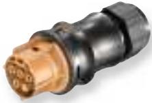
Pluggable connector RST 20i4, 4 pole, screw-in socket part, 50 V, 20 A, for cable diameter 6-10 mm, brown color coding, black housing color; for rigid, for fine-stranded and multi-stranded cables from 0.75 to 4 mm<sup>2</sup>; unassembled with cable screw connection and locking
