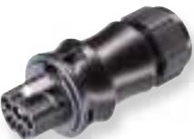
Pluggable connector RST 20i5, 5 pole, screw-in plug part, 250/400 V, 20 A, for cable diameter 10-14 mm, black color coding, black housing color; for rigid, fine-stranded and multi-stranded cables from 0.75 to 4 mm<sup>2</sup>; Degree of protection IP65, IP66, IP67, IP68 (3 m, 2 h); unassembled with cable screw connection and locking, UL/CSA.
