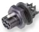
Device connection M25, standard, RST 20i5, 5 pole, screw-in plug part, 250/400 V, 20 A, black color coding, black housing color; for rigid, fine-stranded and multi-stranded cables of 0.75 – 4 mm<sup>2</sup>, 1 connection per pole, with locking, fixed position ensured by flattening of the thread, with thread M25 x 1.5, threaded joint (external), UL/CSA.
