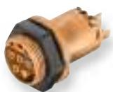
Device connection M25, standard, RST 20i4, 4 pole, screw-in socket part, 50 V, 20 A, brown color coding, brown housing color; for rigid, fine-stranded and multi-stranded cables of 0.75 – 4 mm<sup>2</sup>, 1 connection per pole, with locking, fixed position ensured by flattening of the thread, with thread M25 x 1.5, threaded joint (external)
