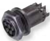
Device connection M25, standard, RST 20i5, 5 pole, screw-in socket part, 250/400 V, 20 A, black color coding, black housing color; for rigid, fine-stranded and multi-stranded cables of 0.75 – 4 mm<sup>2</sup>, 1 connection per pole, with locking, fixed position ensured by flattening of the thread, with thread M25 x 1.5, threaded joint (external), UL/CSA.
