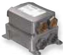
RST compact distributor RST 20i4, 4 pole, 1 input, 3 outputs, AS-i/ 24 V 20 A, brown color coding RST 20i5, 5 pole, 1 input, 3 outputs, 250 / 400 V, 20 A, black color coding with fixing option
