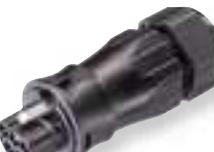
Pluggable connector RST 20i5, 5 pole, screw-in plug part, 250/400 V, 20 A, for cable diameter 13-18 mm, black color coding, black housing color; for rigid, fine-stranded and multi-stranded cables up to 4 mm<sup>2</sup>; Degree of protection IP65, IP66, IP67, IP68 (3 m, 2 h); unassembled with cable
