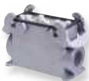
**podis** con surface-mounting housing, 7 pole 20 A with socket insert for **podis** con plug; connection round cable 4 mm<sup>2</sup> via screw terminal; degree of protection IP65; with locking bracket; color: silver gray RAL 7001
