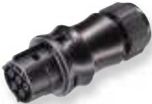
Pluggable connector RST 20i5, 5 pole, screw-in socket part, 250/400 V, 20 A, for cable diameter 10-14 mm, black color coding, black housing color; for rigid, for fine-stranded and multi-stranded cables from 0.75 to 4 mm<sup>2</sup>; Degree of protection IP65, IP66, IP67, IP68 (3 m, 2 h); unassembled with cable screw connection and locking, UL/CSA.
