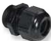
Cable screw connection M 25 x 1.5 for one round cable with outer diameter 13-18 mm; compatible with 75.015.0151.2, 75.018.0051.2 and 75.010.0053.1; color: black, RAL 9005
