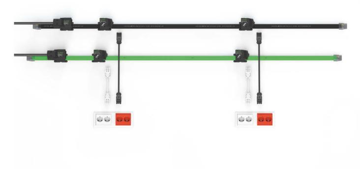
The gesis®NRG flat cables 5G2.5/4 mm<sup>2</sup> can also be used in cable trays thanks to the tap which is routed parallel to the cable. Three-phase power supply up to just before the socket ensures reduced energy consumption. The availability of several cable colors makes it easier to distinguish between networks (NN/IT or general/emergency). The 3-pole, pluggable taps with free phase selection enable flexible load sharing.
