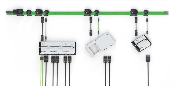
With the decentralized KNX systems gesis®FLEX and gesis®EIB V, the effort involved in cabling for sunshade systems can be greatly reduced. Ideally, these actuators are supplied via a 7-pole gesis®NRG flat cable which provides both three-phase current and the KNX network. For controlling modern SMI drives there is also a corresponding gesis®FLEX KNX SMI gateway.
