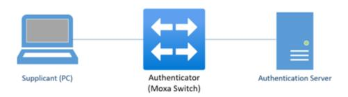
Three components are used to create an authentication mechanism based on 802.1X standards: *Client/Supplicant, Authentication Server,* and *Authenticator*.
